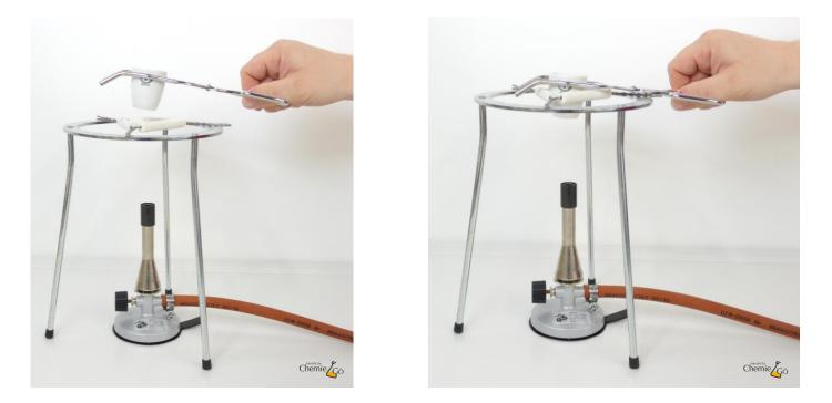
In addition, the crucible tongs can also be used to hold other objects (e.g. metals during annealing).
