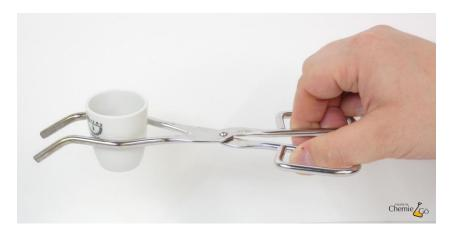
The special oval shape of the gripping parts enables the crucible to be gripped and held securely.
